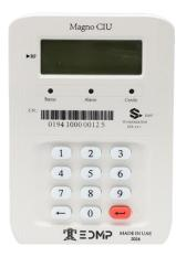
The Magno CIU is a handheld customer interface unit designed for end users to interact with energy meters using the DLMS/COSEM protocol and operate in compliance with **STS/CTS** standards. It enables monitoring of energy consumption and supports prepayment activities. With a slim, lightweight, and durable design, it offers mobility and resilience in various environments, displaying DLMS energy parameters and alarm statuses via keypad input.
